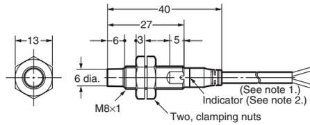
Note 1. 4-dia. vinyl-insulated round cable with 3 conductors (conductor cross section: 0.3 mm<sup>2</sup>; insulator diameter: 1.3 mm); standard length: 2 m
