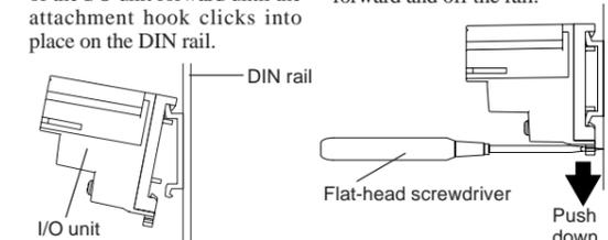
Be sure that the top and bottom faces of the unit are facing the correct direction and the unit is installed in a vertical position. Incorrect installation may prevent heat from dissipating.
