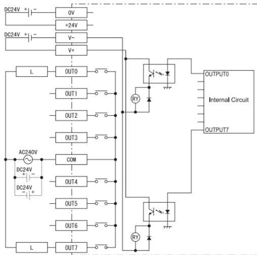
**Note:** The I/O unit's power supply should be separated from the sensor's power supply to prevent the unit from being affected by external noise.
