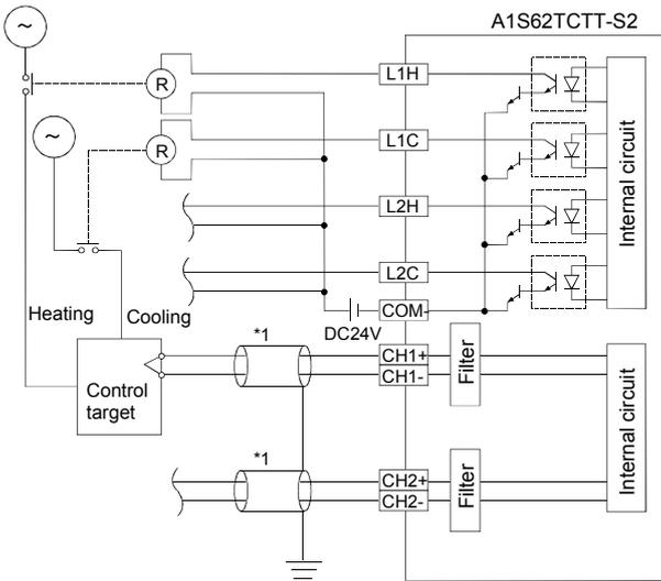
\*1: Always use the shielded compensating conductor for the cable.
