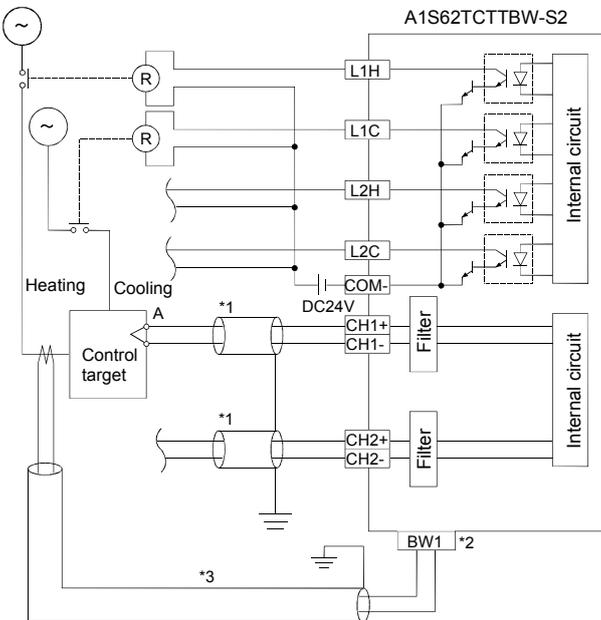
\*1: Always use the shielded compensating conductor for the cable.
