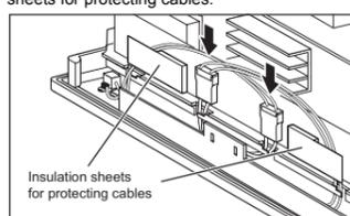
Also assemble the case in the reverse procedure of disassembly. (Tighten the GOT rear fixing screws within the torque range of 0.36 to 0.48N·m). When mounting the case, take care of not biting the cables between the case and the GOT.
