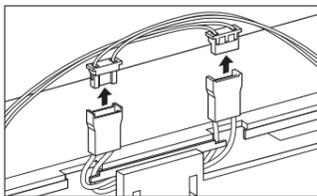
When the GOTs with the following hardware versions are used, remove the cables from the insulation sheets for protecting cables.
