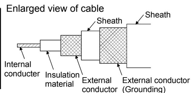
The 5C-2V connector plug is applicable to double-shielded coaxial cable. Connect the 5C-2V connector plug to the coaxial cable inside a double-shielded coaxial cable. Ground the shielded part outside a double-shielded coaxial cable as shown in the above figure.
