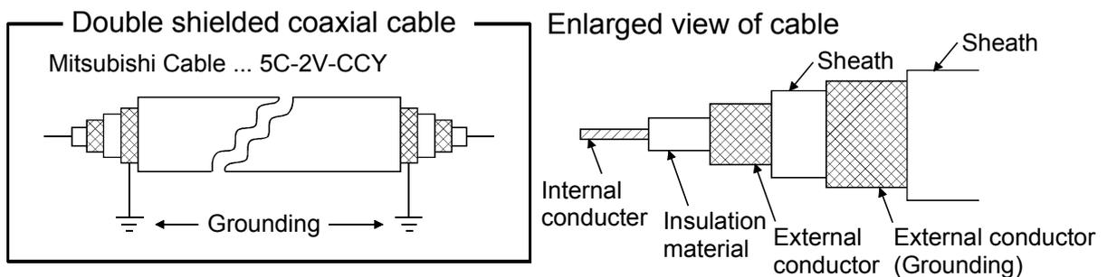
The 5C-2V connector plug is applicable to double-shielded coaxial cable. Connect the 5C-2V connector plug to the coaxial cable inside a double-shielded coaxial cable. Ground the shielded part outside a double-shielded coaxial cable as shown in the above figure.
