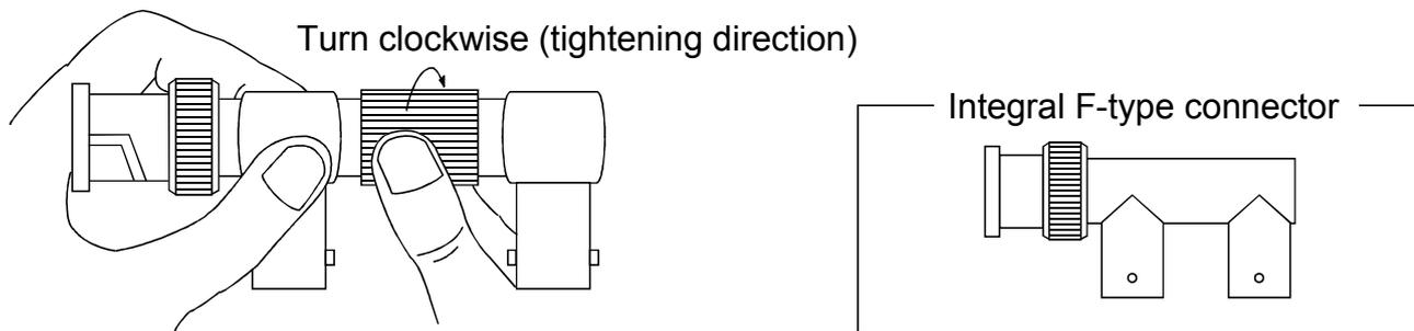
After connecting the F-type connector to the network module, retighten its ring periodically. Retighten it with both hands as shown below.
