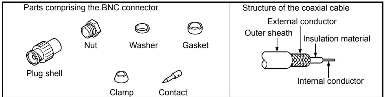
(2) How to connect the BNC connector and the coaxial cable
