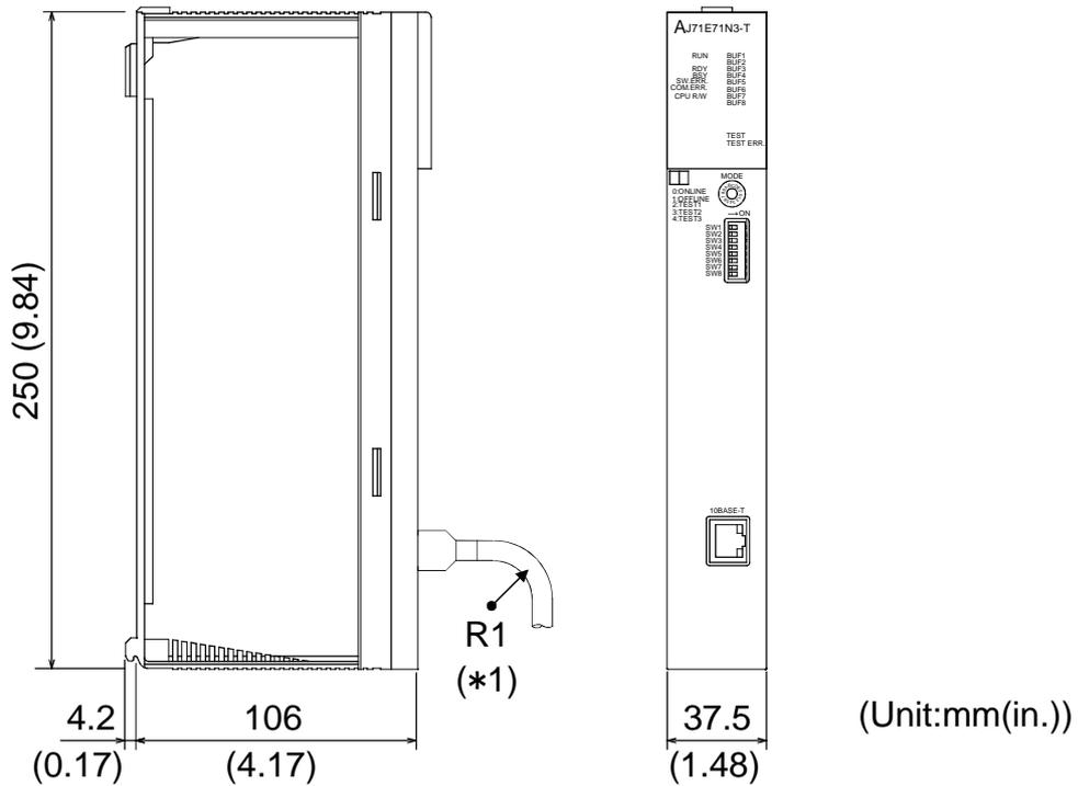
\*1 When connecting the twisted pair cable, make the bend radius (R1: scale value) in the vicinity of the connector to (cable outside diameter × 4) or more.
