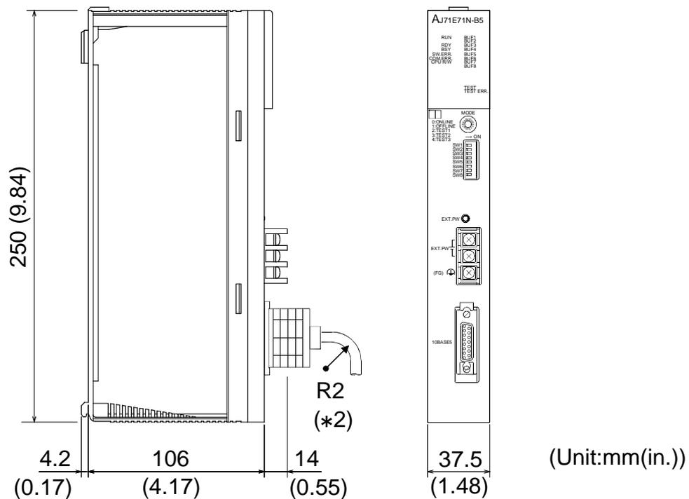
\*2 When connecting the AUI cable, make the bend radius (R2: scale value) in the vicinity of the connector to (cable outside diameter × 4) or more.
