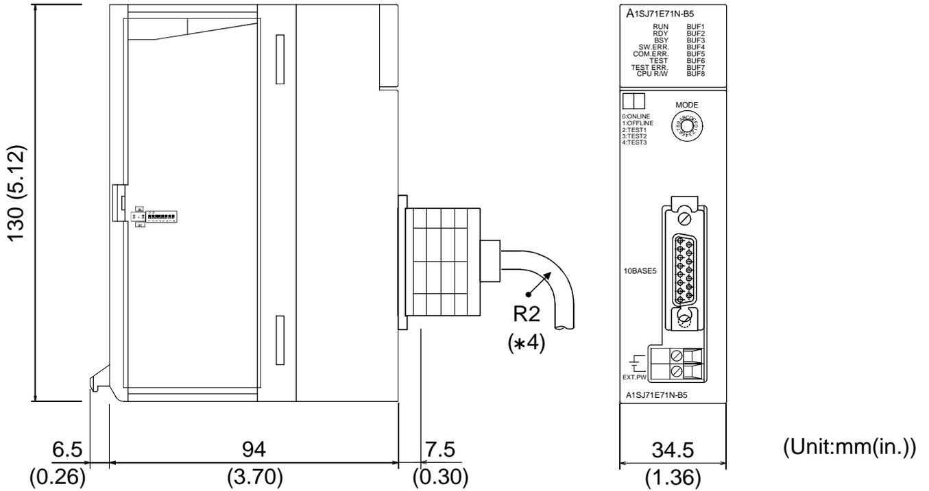
\*4 When connecting the AUI cable, make the bend radius (R2: scale value) in the vicinity of the connector to (cable outside diameter × 4) or more.
