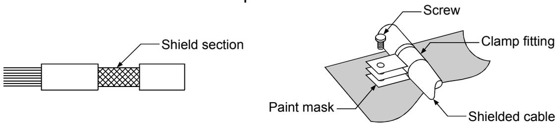
Note) The method of earthing by soldering a wire onto the shield section of the shielded cable as shown below is not recommended. The high frequency impedance will increase and the shield will be ineffective.
