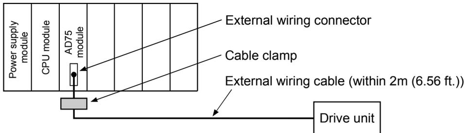
(b) When wiring with cable that exceeds 2 m (6.56 ft.), but is 10 m (32.81 ft.) or less
