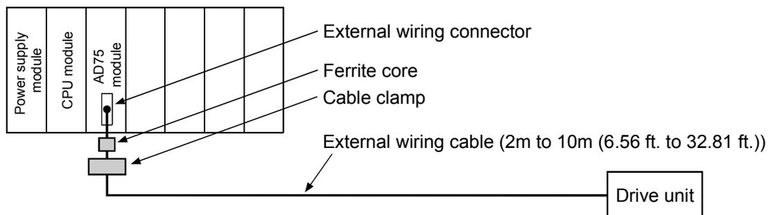
(c) Ferrite core and cable clamp types and required quantities
