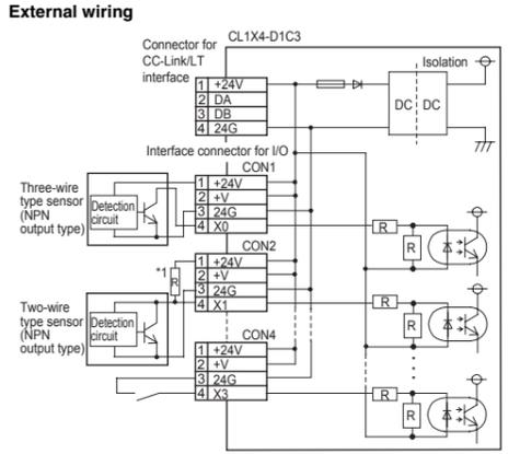
All 24G pin are connected within the module (common). The module power and external power supply for the input are supplied by the power adapter or the dedicated power supply.
