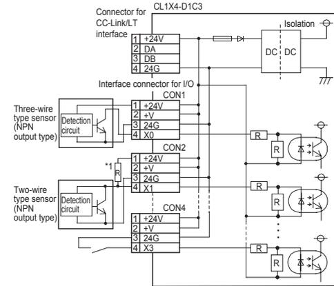
All 24G pin are connected within the module (common).
