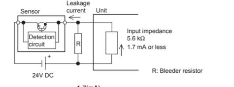
The power capacity W of the bleeder resistor R is as follows:
