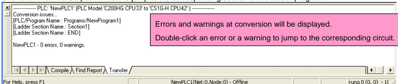
Some instructions can not be converted. Modify the ladder program by referring to *Appendix A. Instructions converted by Change Model on CX-Programmer*.
