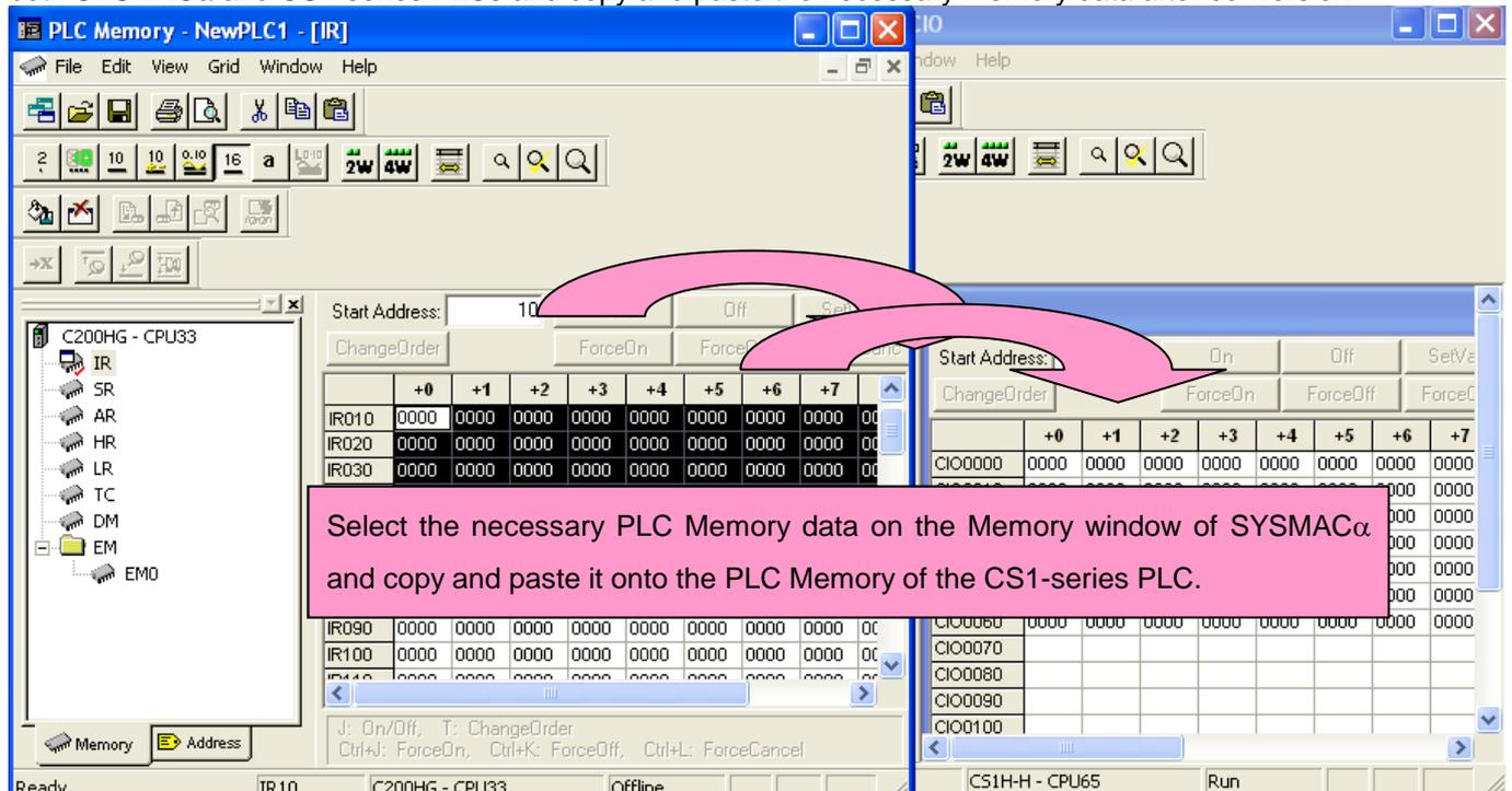
5) The I/O allocation of SYSMAC $\alpha$  series is partly different from that of CS1-series. Refer to *Appendix B. Change of data area allocation* and modify the ladder program.
